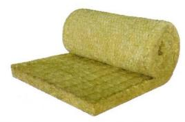
Based on the intended density and thickness, when the coherence of the bulk raw wool is done by curing machine, on the galvanized lace with mesh 1" and 1", according to the standard ASTMC 592, it is sewn by the fireproof wire or thread then rolled, packed and ready to use. Thick type of insulation with thermal resistance about 900 c used under mentioned items, oil, gas, petrochemical, pipes with diameter more than 12 ", duct, turbine, cement industry, steel industry, valve and flange.
